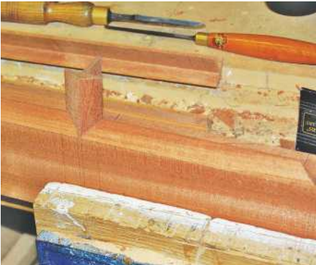
▲ Pic.18 Fitting the glazing bars: Jason used an offcut to get them as close together as possible
